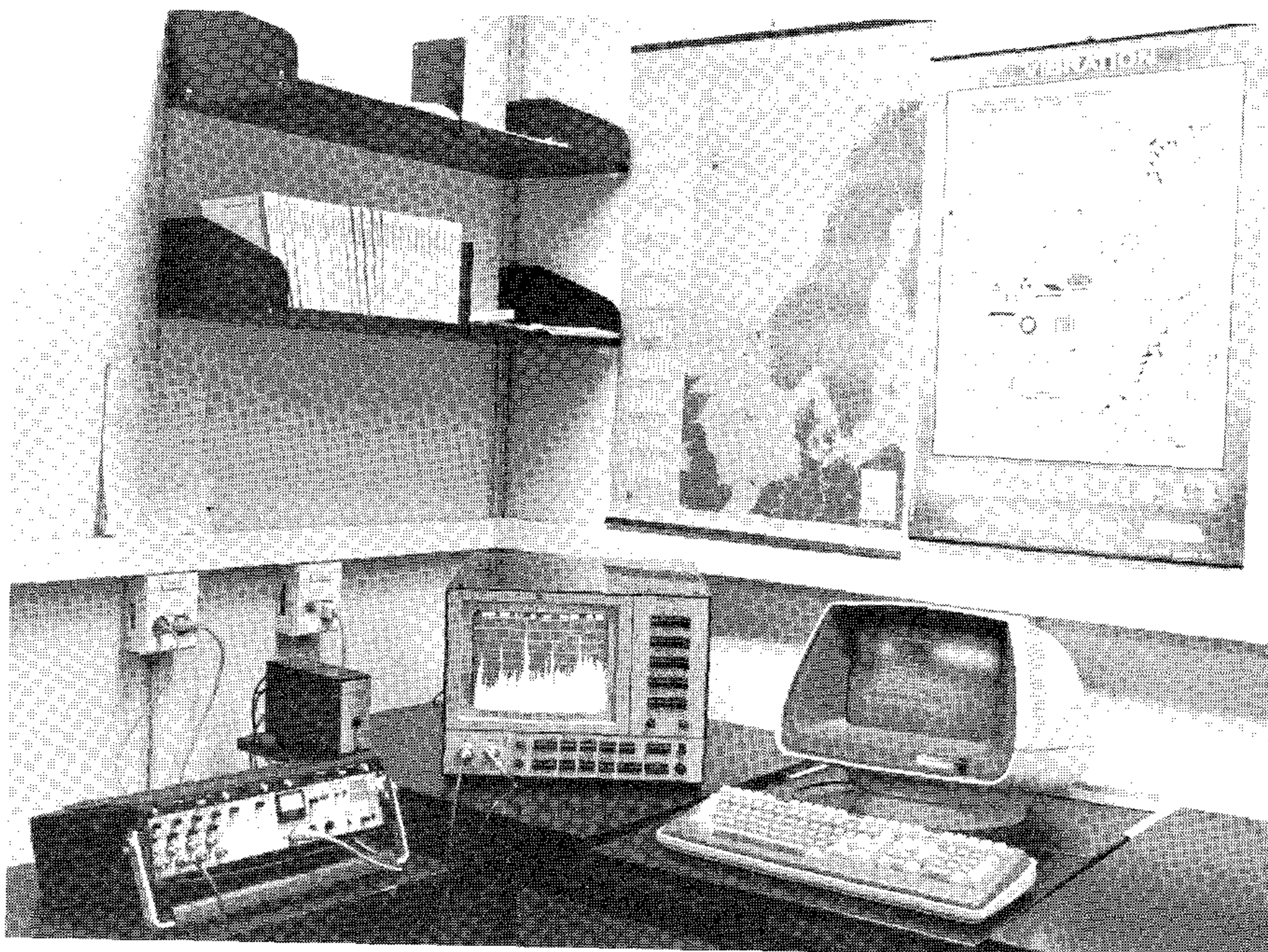
Fig. 2. The computer terminal and FFT Analyzer are placed in the engineer's office next to the central control room. An alarm printer is placed in the actual control room.
